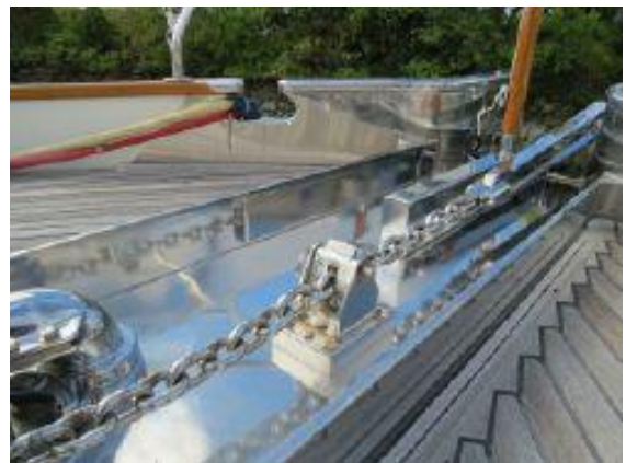
> real chain stop to help windlass
