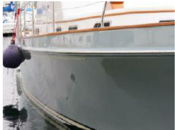
> side note substantial rubbing strake
